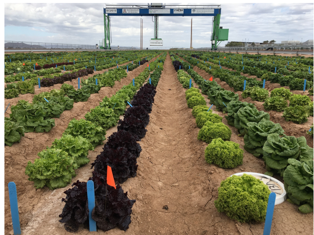
Fig. 1: The gantry system scanning lettuce plants. Different crops are grown under the gantry and scanned daily using various high-resolution sensors and scanners seen hanging below the cross beam and able to move left-to-right as the rig moves forward and back. In the bottom right corner, one can see a GPS marker that we use to develop ground truth for data from this device, as well from the drone.
