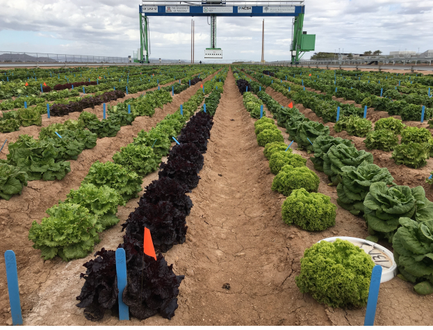
Fig. 1: The gantry system scanning lettuce plants. Different crops are grown under the gantry and scanned daily using various high-resolution sensors and scanners seen hanging below the cross beam and able to move left-to-right as the rig moves forward and back. In the bottom right corner, one can see a GPS marker that we use to develop ground truth for data from this device, as well from the drone.
